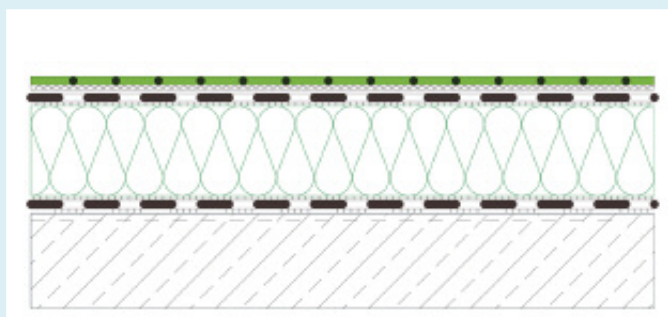
Bonded layer structure
