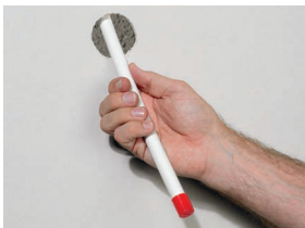
Fig. 23 Always protect pipe ends
