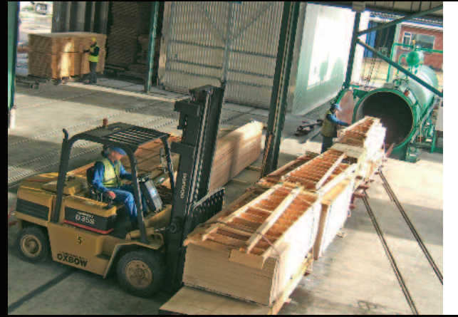
Arch's fire retardant treatment centre - the only one of its type in the UK, operating with ISO 9001 and ISO 14001 accreditations. Treatments involve high pressure impregnation followed by kiln drying/heat curing.
