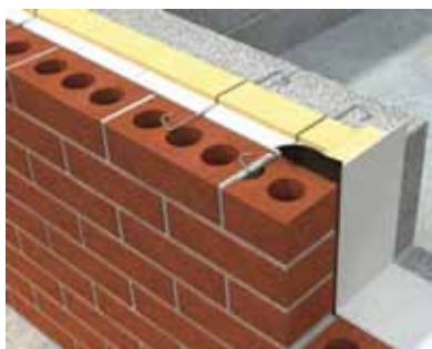
Fig 2 Double wall ties at reveal opening.
