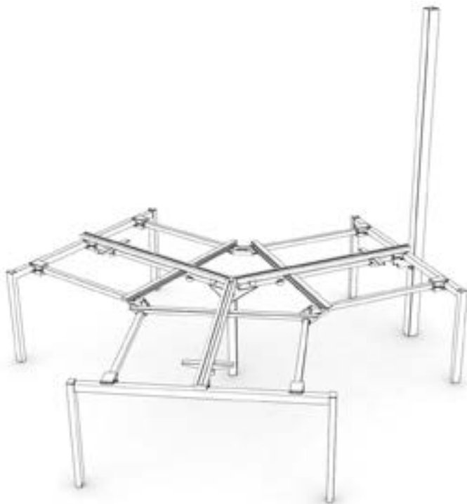
On a 120° Frame, the Ceiling Feed is routed through a Power Pole and then under the worksurface in the same way as used with Single-Sided and Double-Sided Frame.
