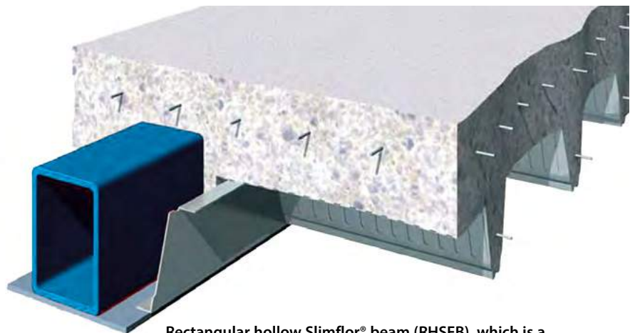
Rectangular hollow Slimflor® beam (RHSFB), which is a rectangular hollow section with a flange plate welded to its lower face (generally used for edge beams).
