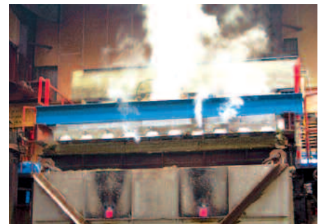
Independent testing of ComFlor® 60 composite floor deck at the Namas certified fire test facility.
