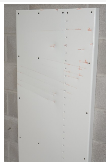
Above, wall mounted NOMS panel before being repeatedly beaten with a four foot long scaffolding pole.
