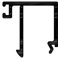
SW467 28mm Internal Glazed Bead EXTERNAL PERIMETER 169mm
