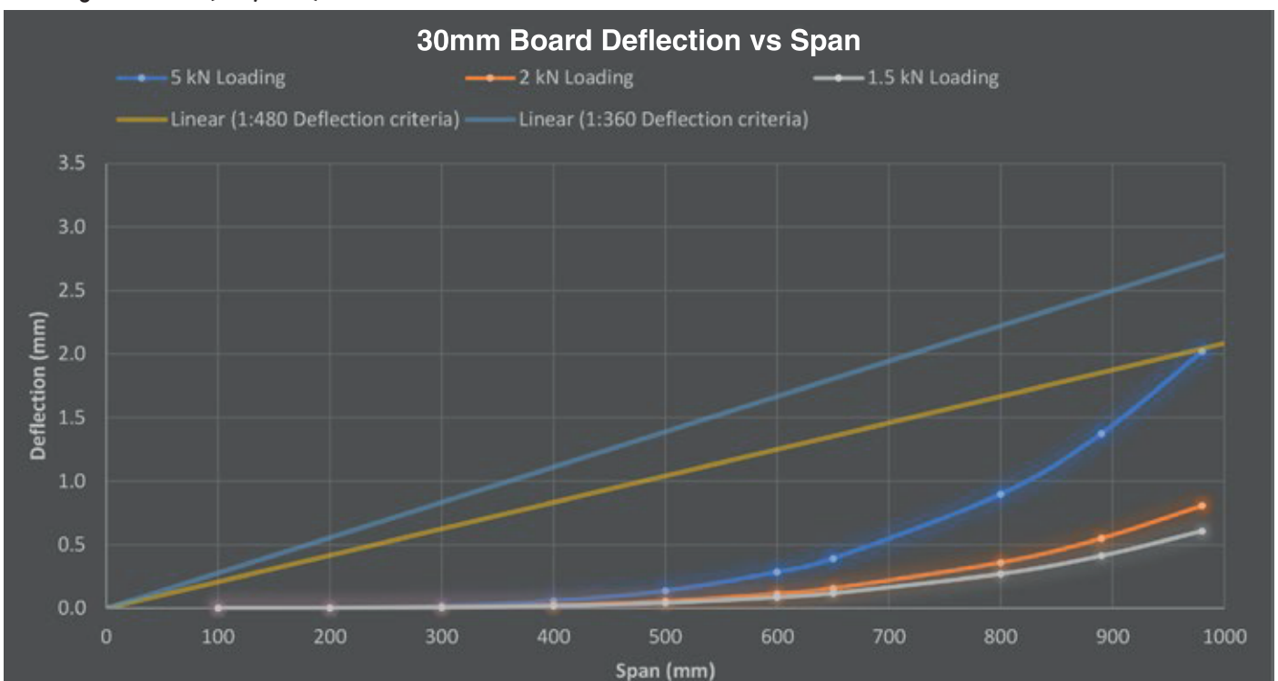
Loading deflection (kN / m 2 )
