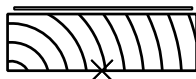
Batten_Std Standard softwood ground. For cill & right jamb. Mirror for head & left jamb.
