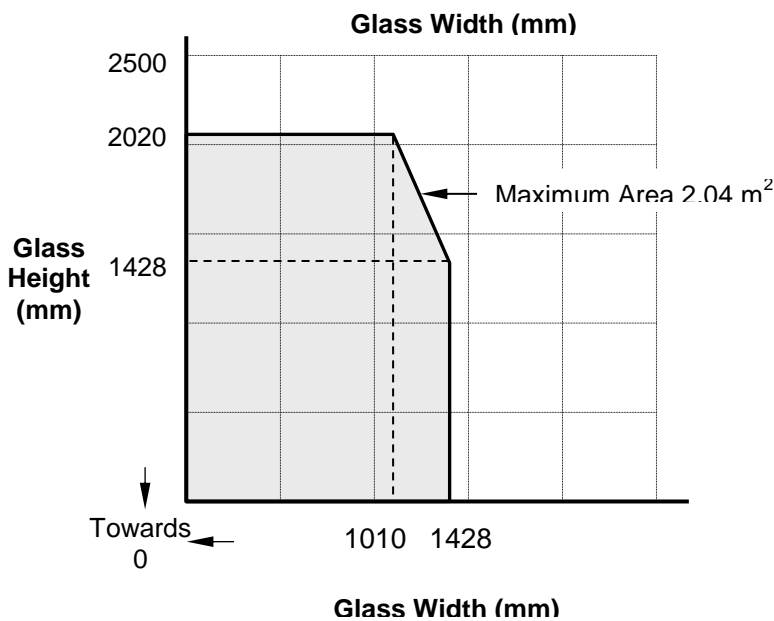
Figure 4. Maximum Permitted Pane Dimensions 60 minutes Integrity
