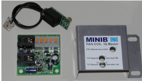
Fig. of the module DC-BLOK with the temperature sensor and connecting cable
