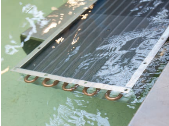
Air under water testing
