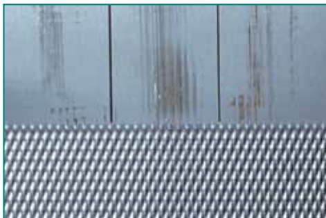
Test sample illustrating the scratch resistance properties of Rimex's Patterned Finishes as compared to a satin polished finish.
