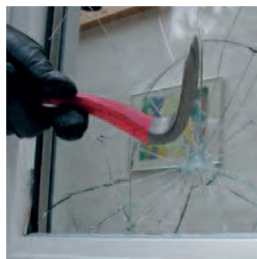
7. The relatively long time it takes to break a laminated pane will discourage even the most persistent burglar.
