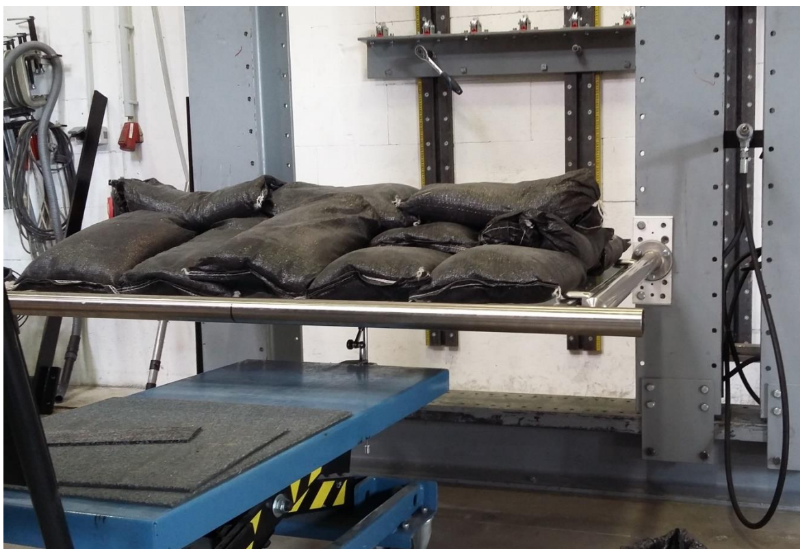
Typical arrangement for application of uniformly distributed load applied to the balustrade system
