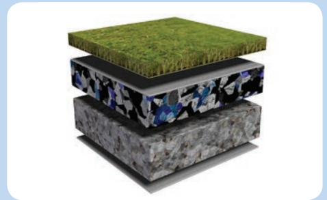
Play Turf Safer Impact - Recycled foam shock pad on top of 50mm stone & geo textile membrane
