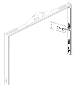
swivel VESA monitor mounting bracket. maximum weight 24kg
