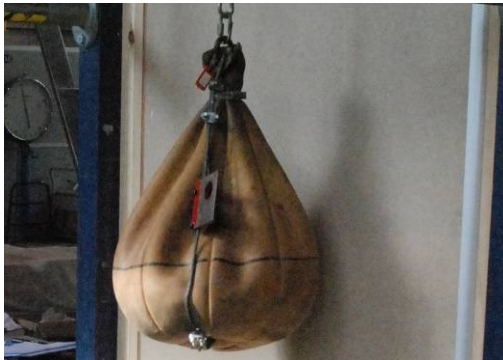
Figure 3: 300N heavy body impact test
