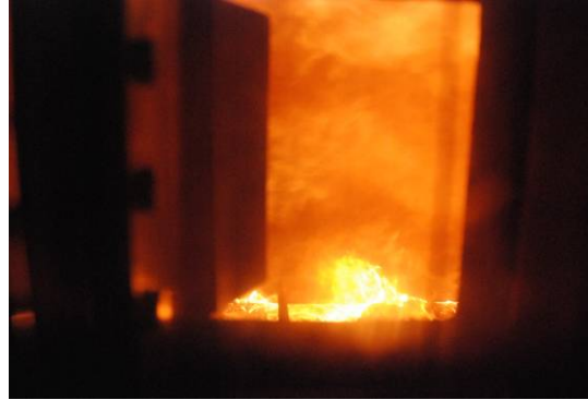
Figure 2: view inside furnace at 25mins, temp 825°C
