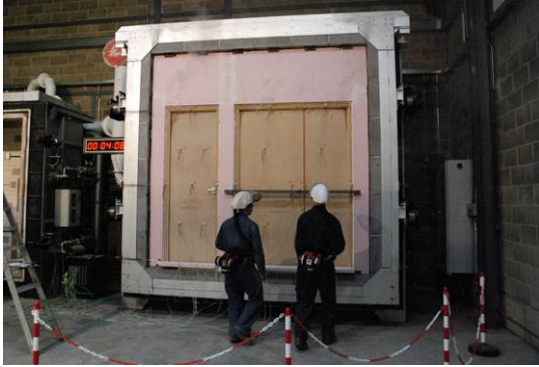
Figure 1: FD30 test in progress
