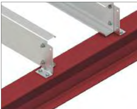
Oversail/top cleat connection between C-section secondary beams and hot rolled primary beam
