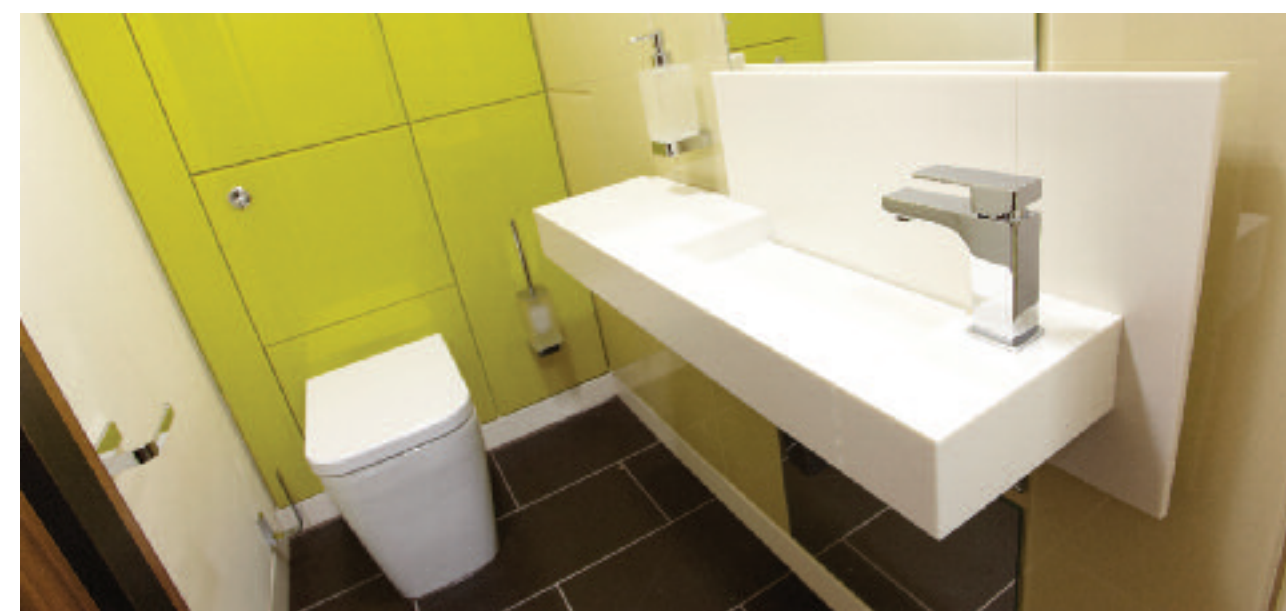
Back-painted glass for WC and wall panelling. WC panelling in RAL1012 and washhand basin in RAL1015.
