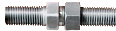
Screwing the adapter brings the rebars together up to the limit stop. A locknut is used for fixing the assembly.
