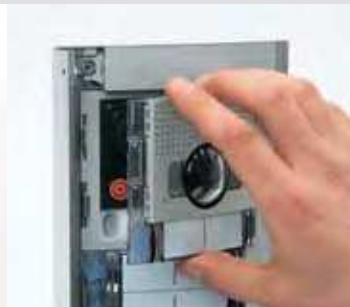
3 Loosen the clips and slip off the front plate
