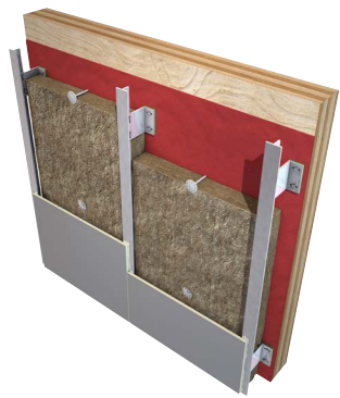
Cross laminated timber with cladding
