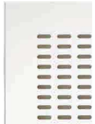
Tangent, 4 x 14 mm, 10/20 mm c/c Perforation: 21.3%
