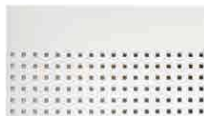
Micro, 3 x 3 mm 8.3 mm c/c Perforation: 10%
