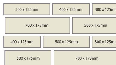
5 size mixed pack, unit sizes and quantities per layer, as supplied.
