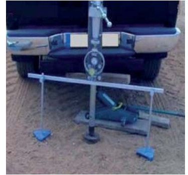
CBR Testing being carried out on site
