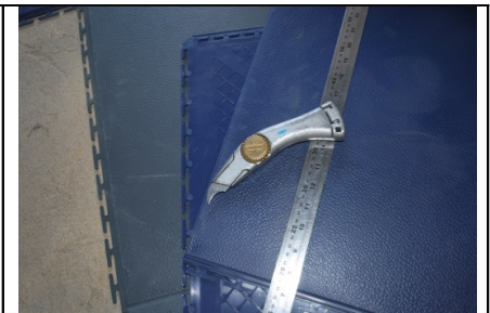
Stanley knife with concave blade
