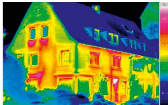
Pictures taken with the thermal imaging camera help to detect thermal bridges on the house. Photo: Association of Private Builders e. V./ Federal Association of German Building Material Specialist Distribution e. V.
