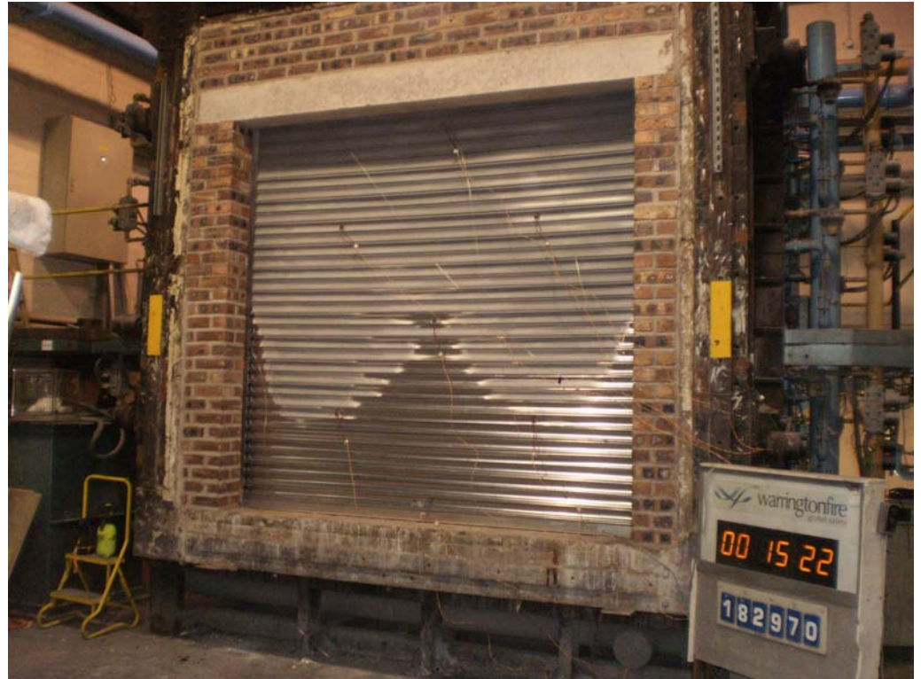
The unexposed face of the test construction after 15 minutes of testing
