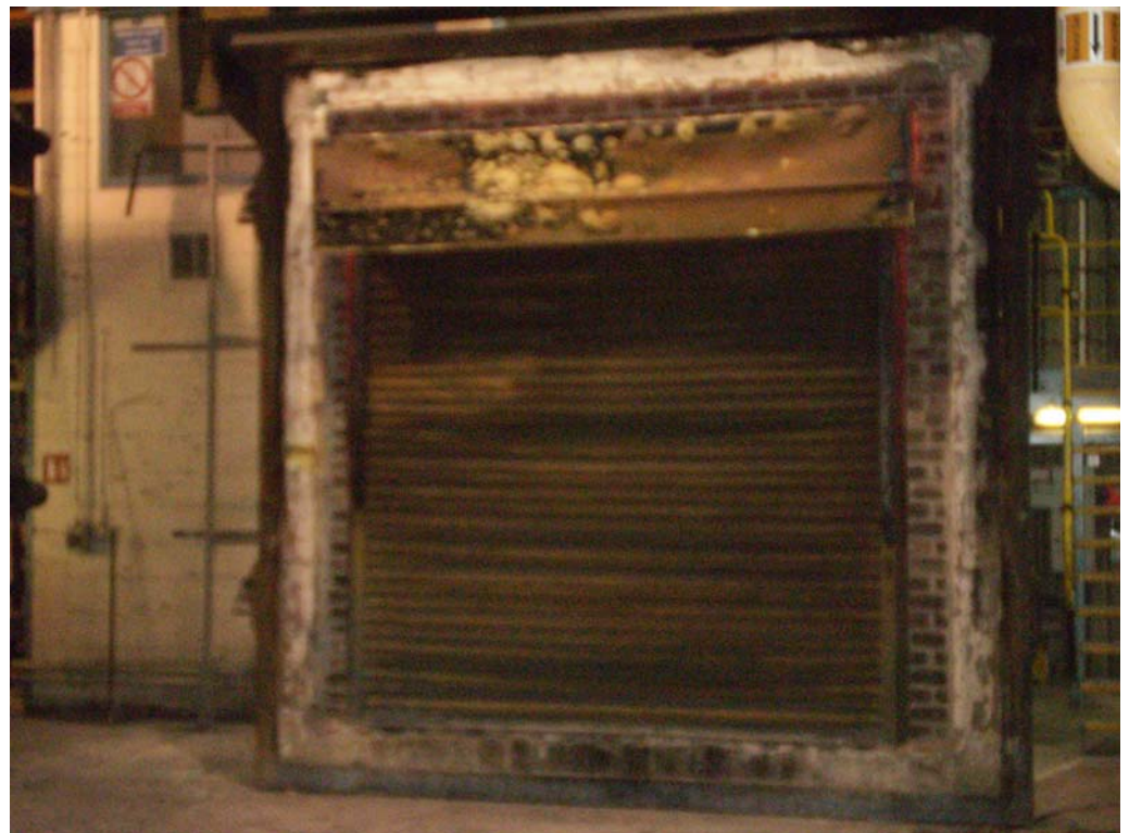
The exposed face of the test construction immediately after testing
