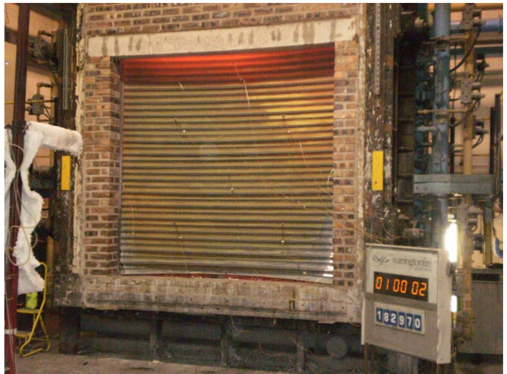
The unexposed face of the test construction after 60 minutes of testing
