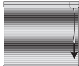
To Raise: Pull the wand straight down with short strokes.
