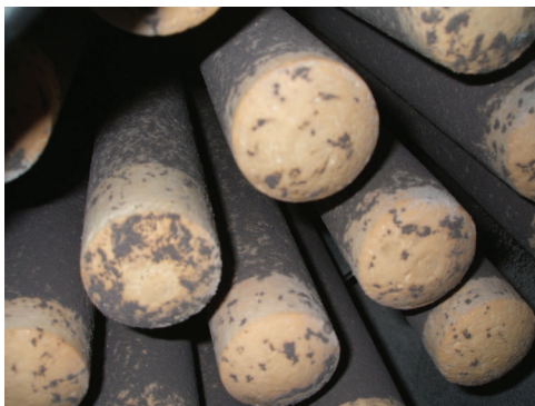
Ceramic filters after cleaning process
