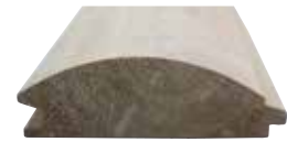
44mm x 144mm (covers 132mm) x random lengths Loglap Use Class 3
