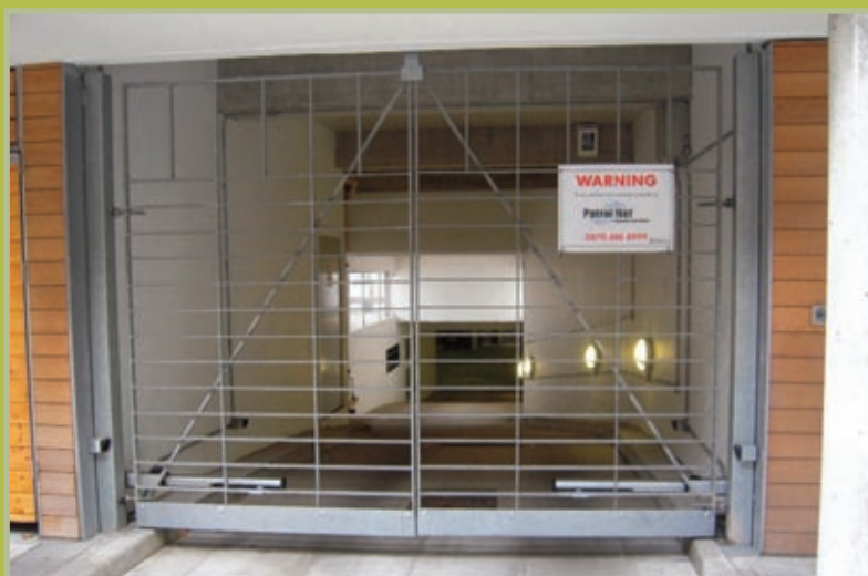
Galvanised double swing gates, automated by hydraulic rams. Manufactured to Architects design
