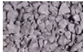
Upper layer 100mm depth 5mm-20mm clean, crushed with well defined edges BS EN 13242:2002
