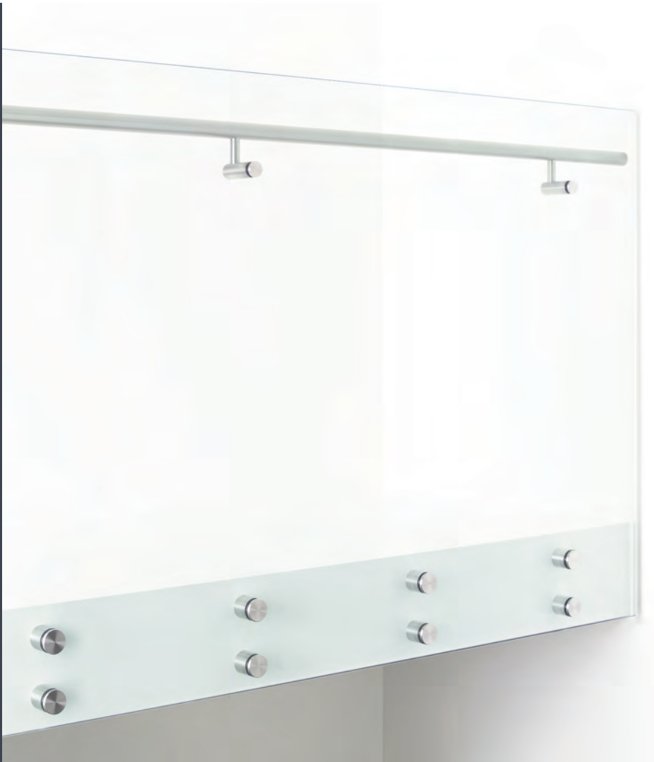
S.4G.6B.CG.15* Satin Polished Stainless Steel 38mm diameter top rail with offset stem brackets bolted to 15mm toughened clear structural glass panels with flat arrisred and polished edges all round, 2-point side fixed at appropriate centres with Satin Polished Stainless Steel bosses. * Transpose choice of glass thickness to suit application - see technical table on page 11.
