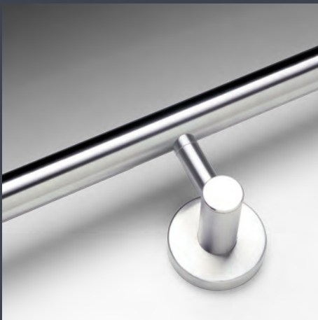
SS.1C.38 Satin Polished Stainless Steel handrail connected at maximum 1200mm centres to Stainless Steel stem brackets with concealed fixings.
