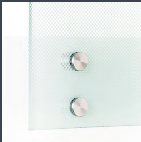
6B Boss Fixing Satin Polished Stainless Steel 50mm diameter bosses with concealed bolts clamping dot matrix screen printed clear glass. Other screen printed options available upon request.
