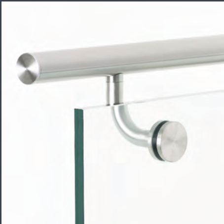
S.4K Satin Polished Stainless Steel 38mm diameter toprail with offset bend brackets bolted to glazing at appropriate centres.
