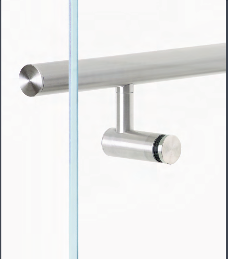
S.4G Satin Polished Stainless Steel 38mm diameter toprail with offset stem brackets bolted to Low Iron clear raised glass at appropriate centres.
