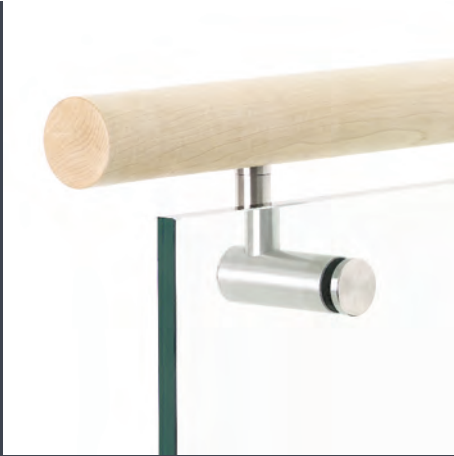
H.4G Polished Maple Hardwood 50mm diameter toprail with offset stem brackets bolted to glazing at appropriate centres.
