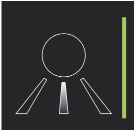
2. Symmetric Orientation – Downward Facing Provides even illumination from the centre of the handrail, ideal for divider rails to wide entrance steps and ramps.
