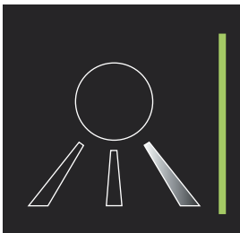
3. Asymmetric Orientation – Backward Facing Provides ambient lighting, bathing the wall in light - RGB LED's create contrasting and colour changing effects. Any angle can be specified.
