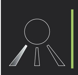
1. Asymmetric Orientation – Forward Facing Provides walkway illumination, highlighting the route of travel and reducing emergency lighting requirements. Any angle can be specified.
