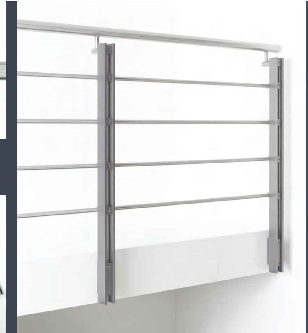
SN.4G.5E.6G.X4 Satin Polished Stainless Steel toprail connected with offset stems to Tungsten NyMet® coated fin side fixed twin flat uprights at maximum 1400mm centres with 4 x 22mm diameter offset midrails.
