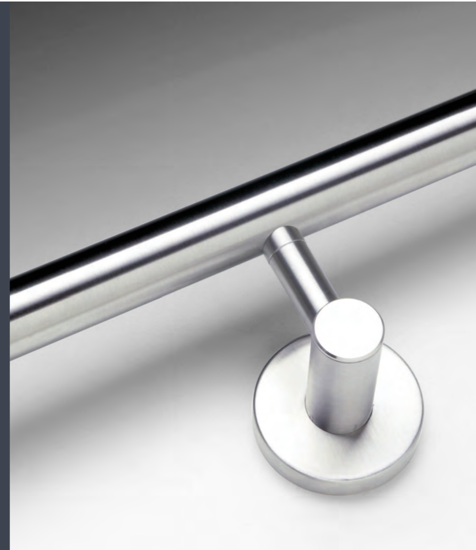
SS.1C Satin Polished Stainless Steel handrail connected at maximum 1200mm centres to Stainless Steel stem brackets with concealed fixings.
