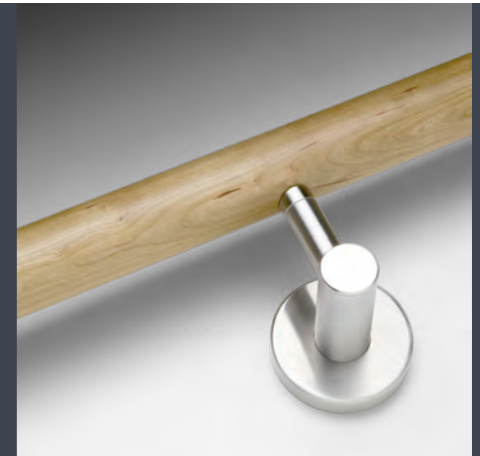
HS.1C Polished Cherry Hardwood handrail connected at maximum 1200mm centres to Stainless Steel stem brackets with concealed fixings.
