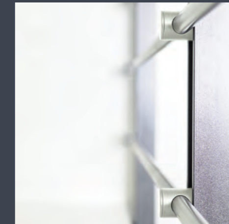
SN.4G.5E.6G.X4 Satin Polished Stainless Steel toprail connected with offset stems to Tungsten NyMet® coated fin side fixed twin flat uprights at maximum 1400mm centres with 4 x 22mm diameter offset midrails.
