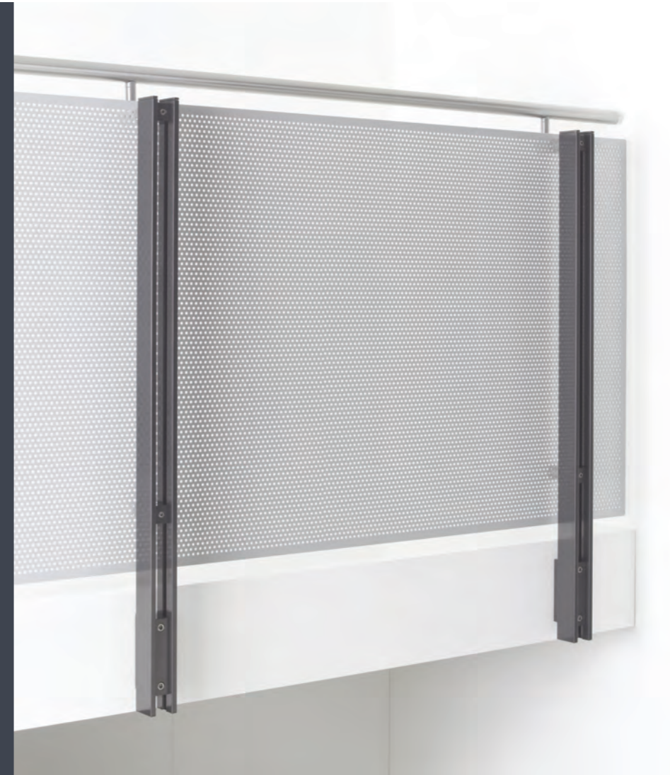
SN.4H.5C.6G.PC6 Satin Polished Stainless Steel toprail connected with offset stems to Gun Metal NyMet® coated fin fixed twin flat uprights at maximum 1400mm centres with offset panel holders supporting 3mm thick NyMet® coated Mild Steel infill panels.
