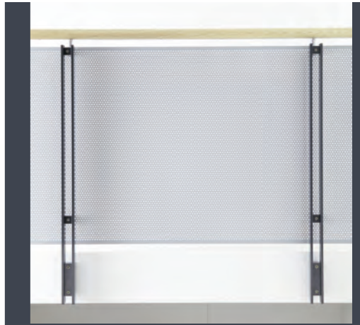
HN.4H.5C.6G.PC6 Polished Maple Hardwood toprail connected with offset stems to Gun Metal NyMet® coated fin fixed twin flat uprights at max 1400mm centres with 3mm thick NyMet® coated Mild Steel infill panels.
