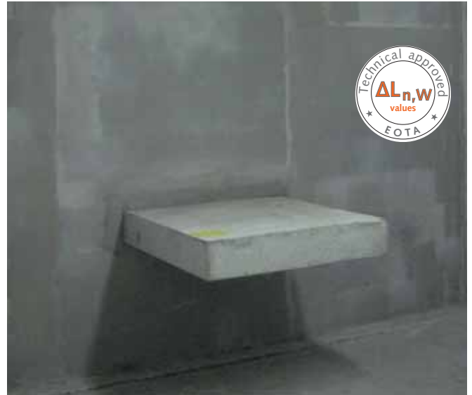
Test setup according to EN ISO 10140 with built-in element
