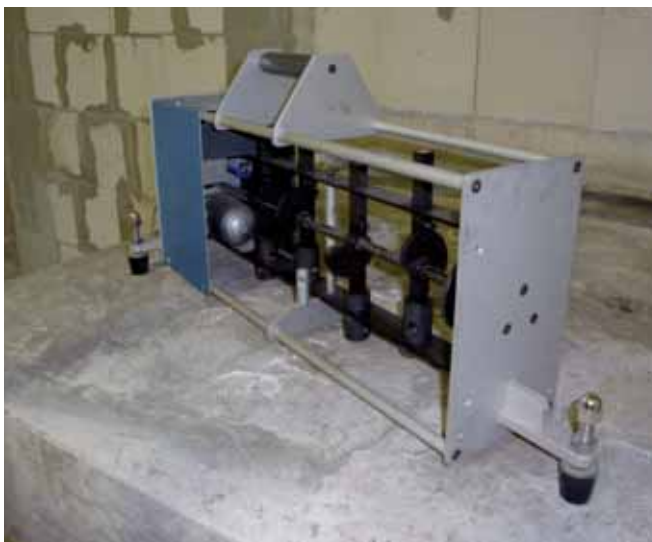
Standardised tapping machine according to EN ISO 10140
