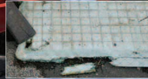
Trench-Guards do not splinter on the edge like fibreglass panels do.
