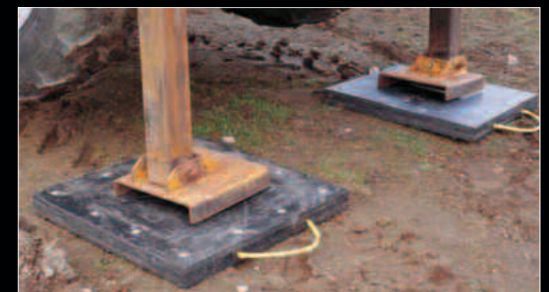
Outrigger Pads prevent ground damage by excavator jack legs.
