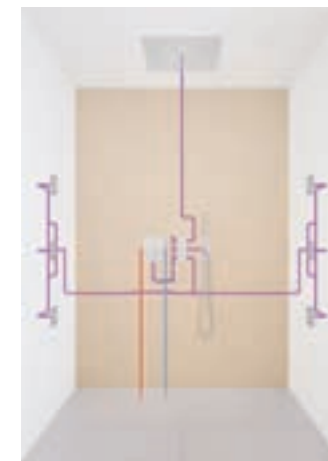
Central thermostat mixer in the shower with 3-way concealed valves Grotherm F
