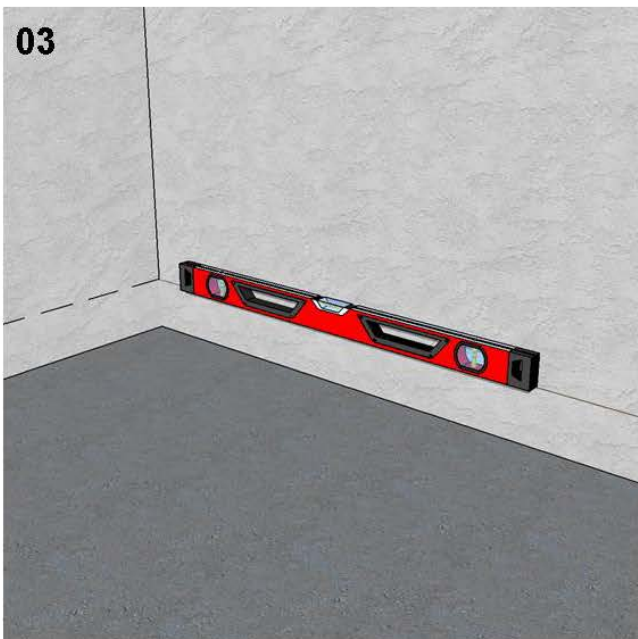
03 - Using a string or chalkline and spirit level set out a horizontal setting out line to one edge, Set the string line at distance 'A' above the highest edge, in line with the top of the paving slabs
