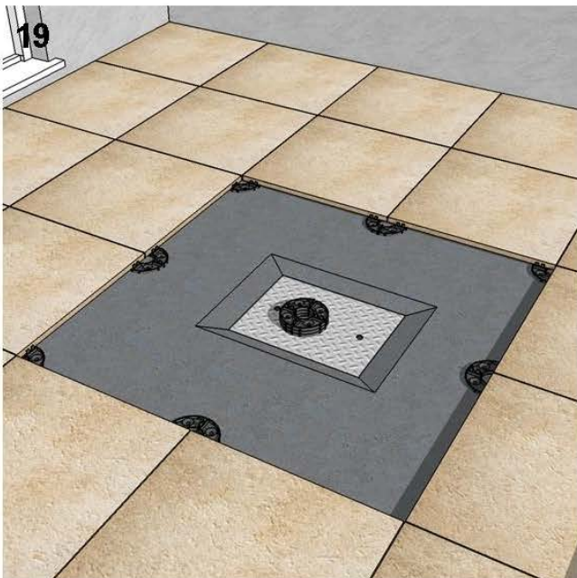
19 - For recesses, recessed manholes/drains or level changes, you may require to stack up to a maximum of 2N° PS20 paving supports and 3N° LGH3 shims, alternatively NM 1-5 pedestals can be employed for recesses greater than 36mm deep. See our full range of accessories so that you select the appropriate pedestals to suit your application.
