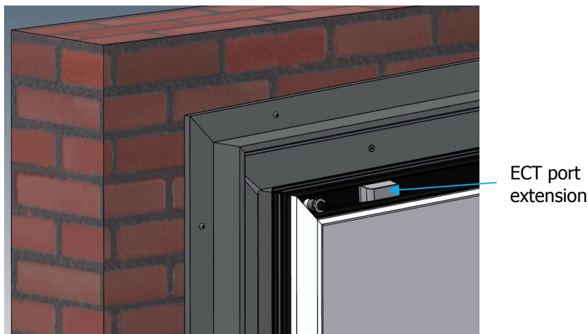
Figure 16 – ECT port extension
