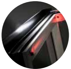
built in infra red proximity detector
