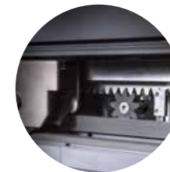
rack and pinion drive system with large diameter carriage wheels
