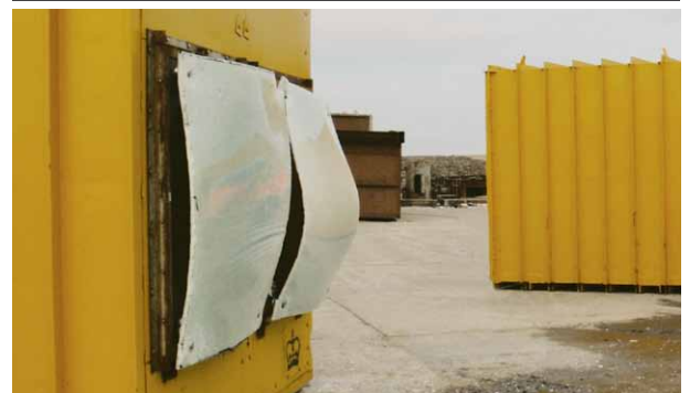
Test Rig: showing post-blast impact
