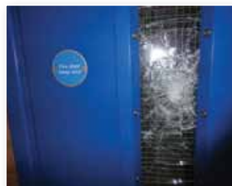
Axe attack on the anti-vandal 3tiervision™ panel. The fire door is still able to function with no breach to the inner section of fire resistant glazing.
