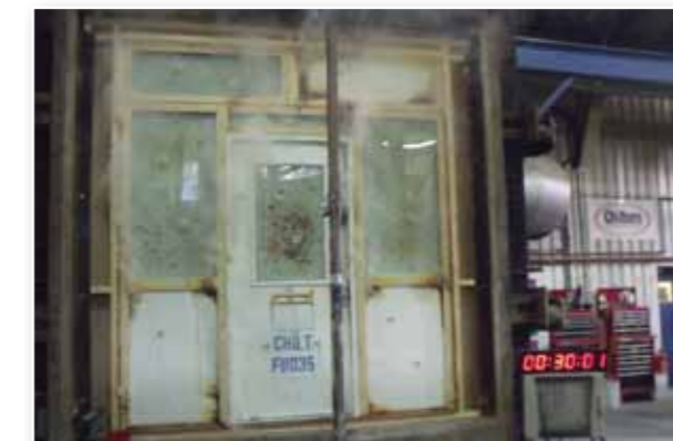
Fire test after 30 minutes
