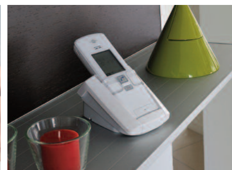
Handset with mains powered charging base, table mounted
