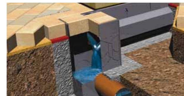
FacadeSlot with Outlet Box
